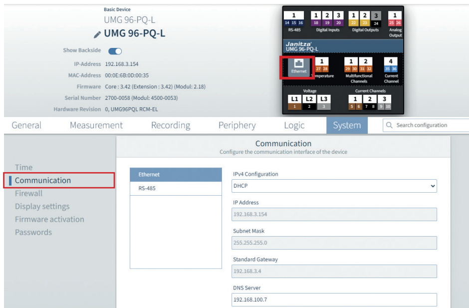
Fig. Ethernet configuration via the GridVis® software, Ethernet interface selected
