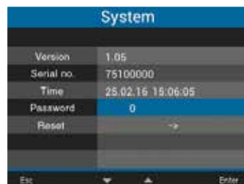
Display of device data, password assignment and option to reset the device
