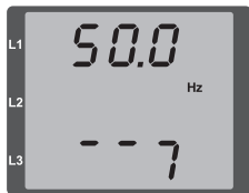
Fig. Display of the mains frequency (50.0) and the direction of the rotary field
